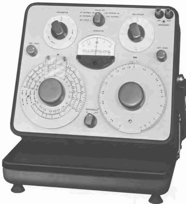
FIGURE 5 The General Radio Type 1650-B Impedance Bridge.
